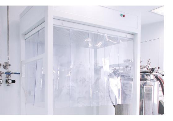
The movable box is a corpus for mobile device equipped with circulating units, which is used (together with flexible screens, which increase the protection of the product) to set up a closed workplace with uniform airflow, lighting and the required class of cleanliness.
